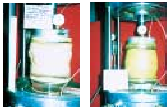
Fig. 9. Triaxial testing of sand samples. The interlocking aggregations are clearly visible as bulges in the sand sample on the left containing mesh element inclusions. The sand only sample on the right shows no evidence of aggregation at high strains.
